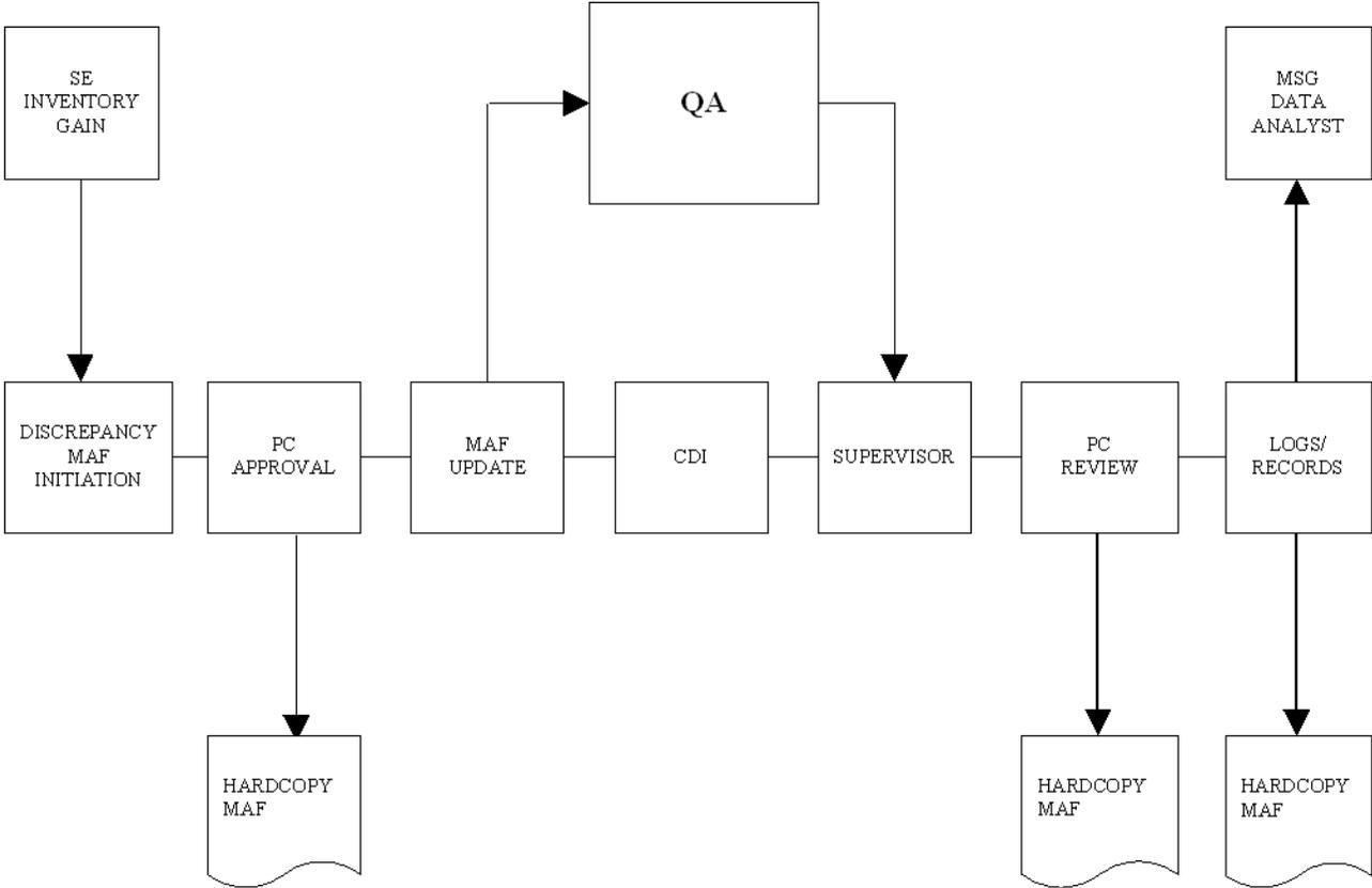
Figure 16-8: On-Equipment Work Documentation Flow
