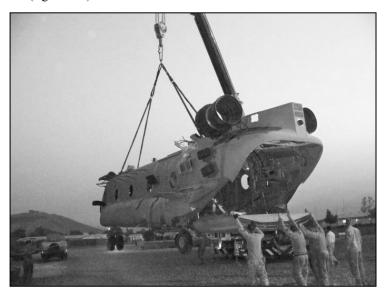
Figure 3-3. Recovery by crane
