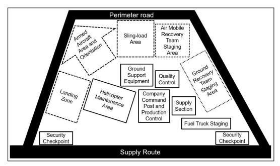
Figure 2-4. Helicopter maintenance collection point
