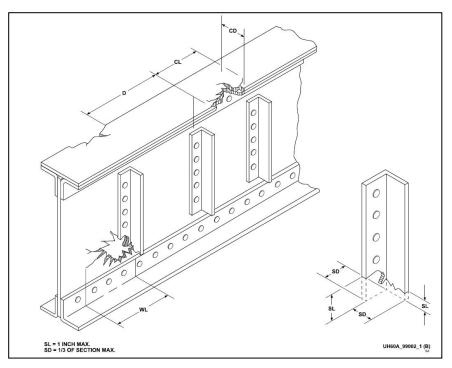
Figure 2-2. Inspecting damage to aircraft airframe
