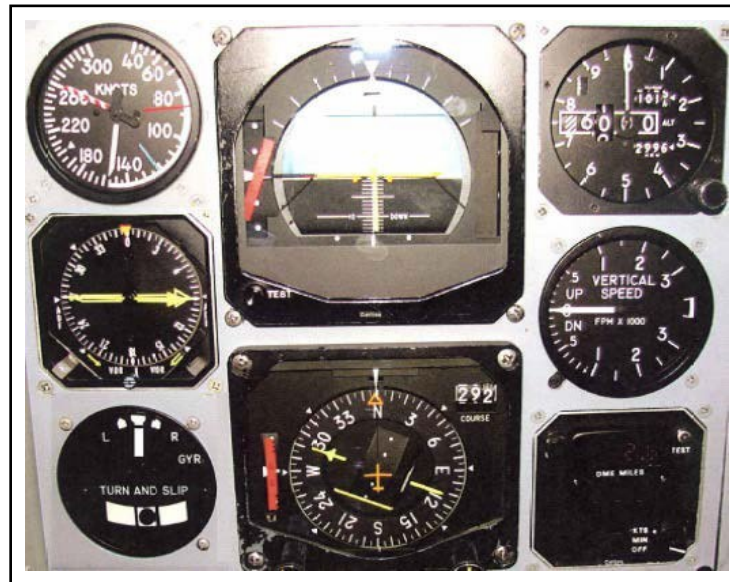
Figure 3-1. Pitch attitude and airspeed in level flight
