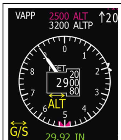
Figure 1-7. UH60M digital barometric altimeter
