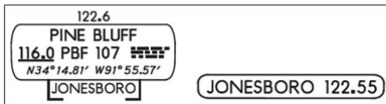
Figure 4-6. Remote communications outlet
