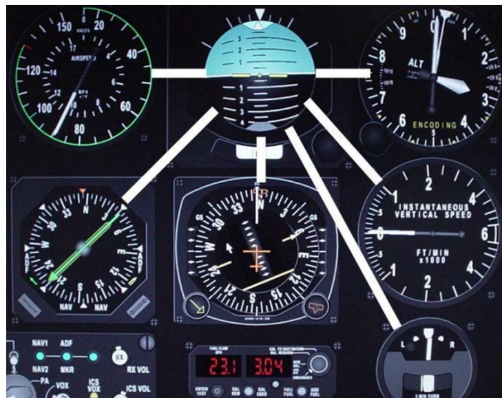
Figure 2-7. Analog cross-check pattern
