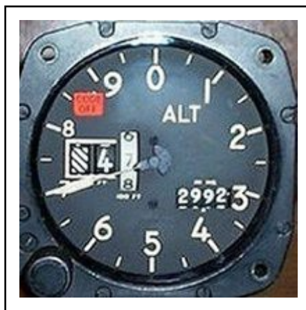
Figure 1-6. Encoding altimeter with a malfunction
