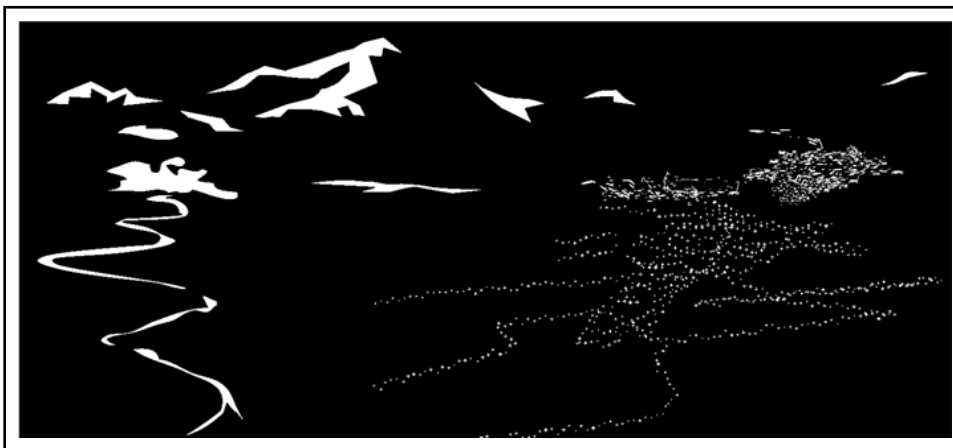
Figure 9-2. Typical light pattern for airport identification
