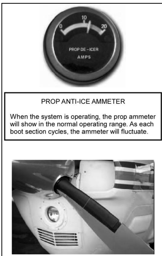
Figure 8–6. Propeller ice control
