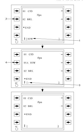
Figure 3C-34. Inserting and Deleting Intermediate Flight Plan Waypoints
