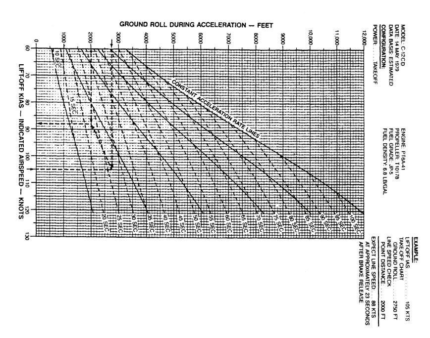
Figure 7-24. Line Speed Check During Takeoff Ground Run
