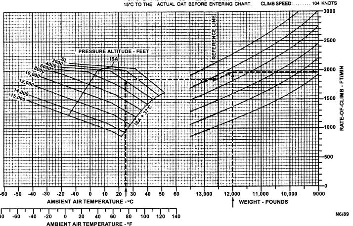
Figure 7-26. Climb Two Engines – Flaps 40%
