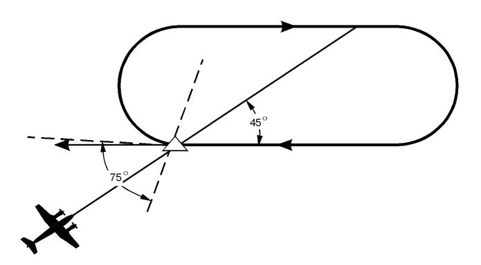
Figure 3C-74. Teardrop Entry Into a Holding Pattern
