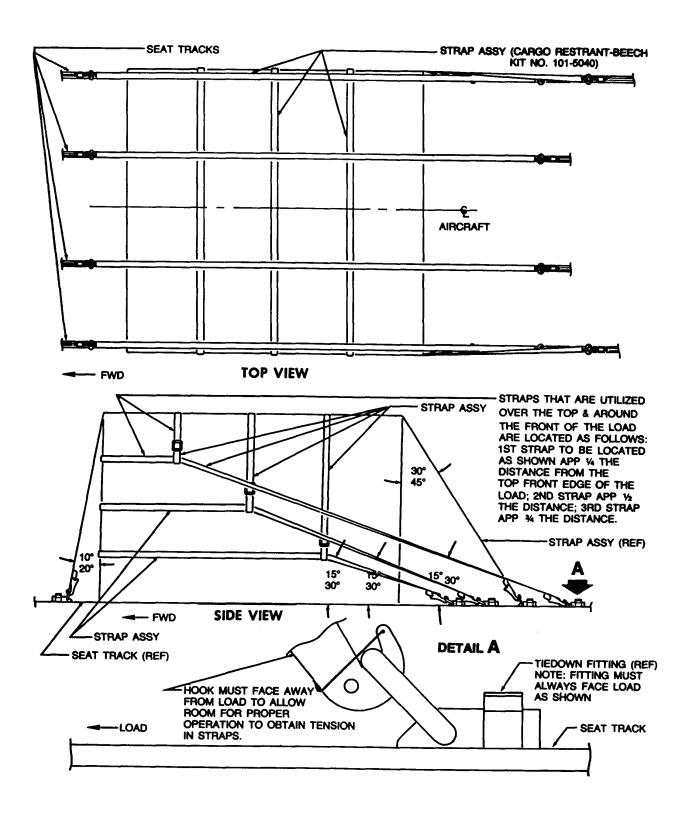
Figure 6-9. Cargo Restraint and Tiedown Method
