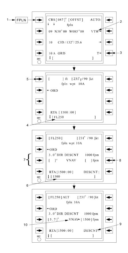
Figure 3C-56. Entry and Display of VNAV Parameters
