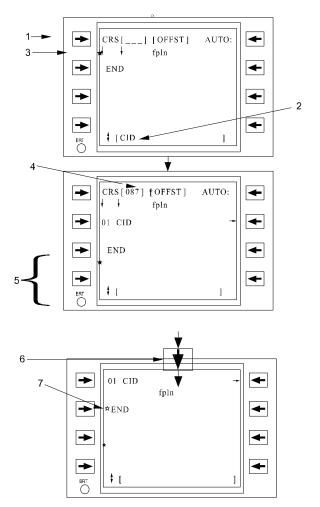
Figure 3C-33. Inserting Flight Plan Waypoints in Sequence
