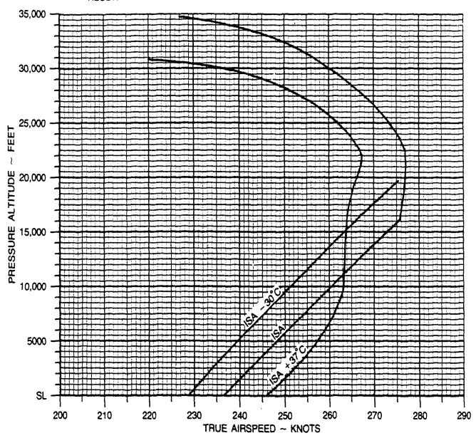
Figure 7A-42. Normal Cruise Speeds, 1700 RPM
