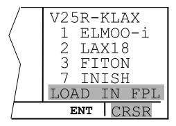
Figure 3-60. Loading the Approach
