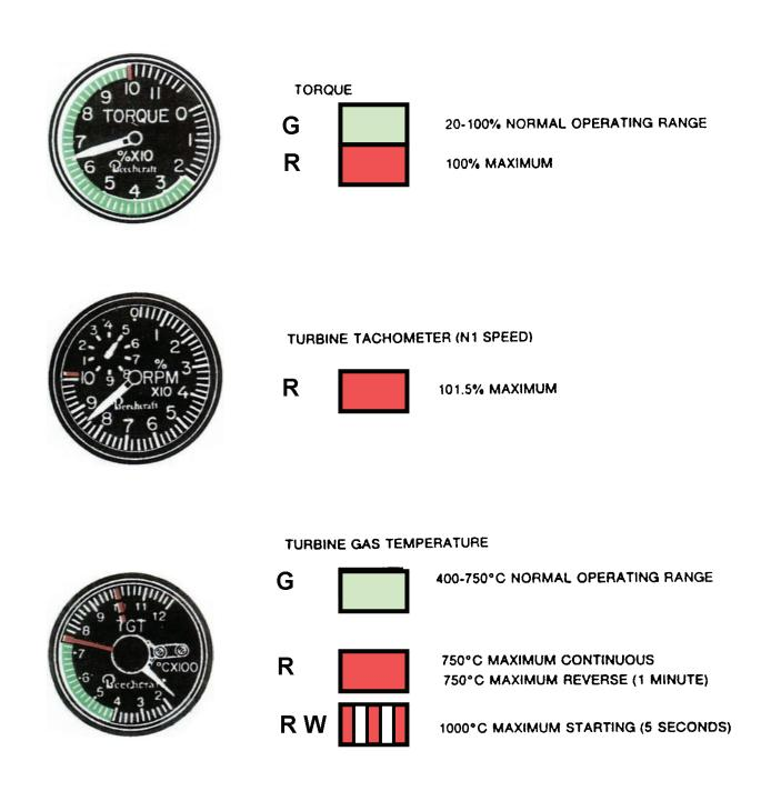
Figure 5-1. Instrument Markings and Operating Limits C D (Sheet 1 of 7)
