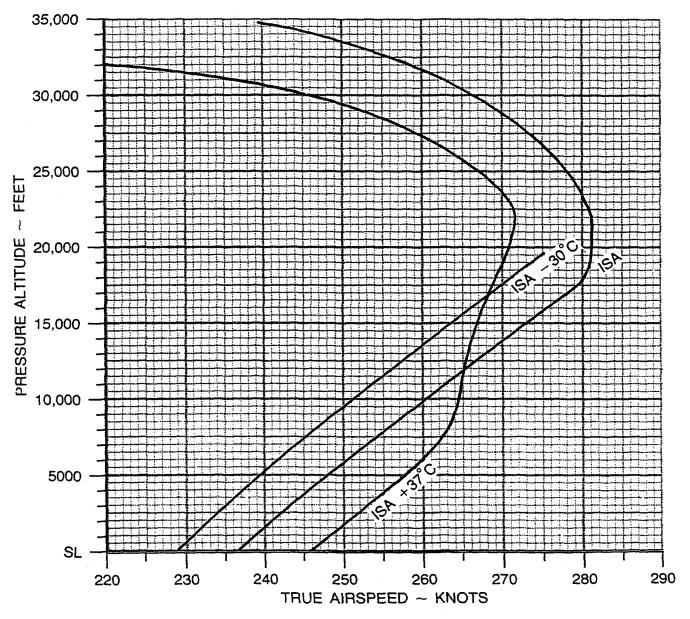
Figure 7A-54. Maximum Cruise Speeds, 1700 RPM
