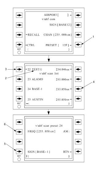
Figure 3C-127. Scan Preset Page Access and Usage
