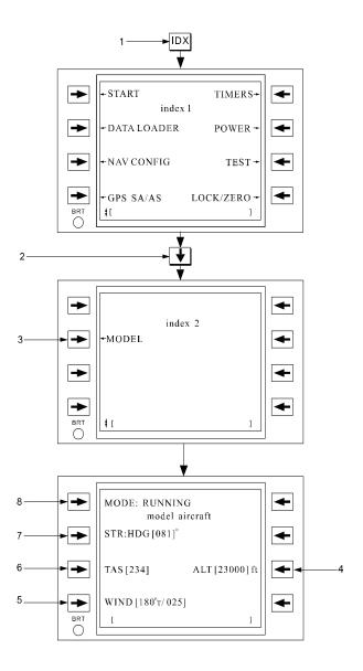
Figure 3C-141. Model Aircraft Page Access and Function
