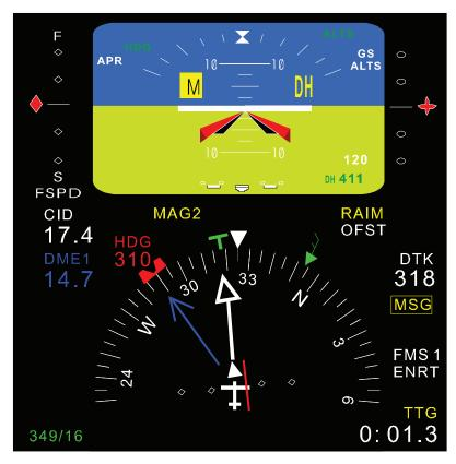
Figure 3C-9. Primary Flight Display Mode Display
