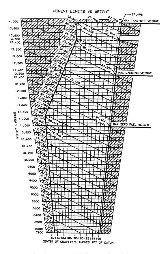
Figure 6-8. Center of Gravity Limitations Above 12,500
