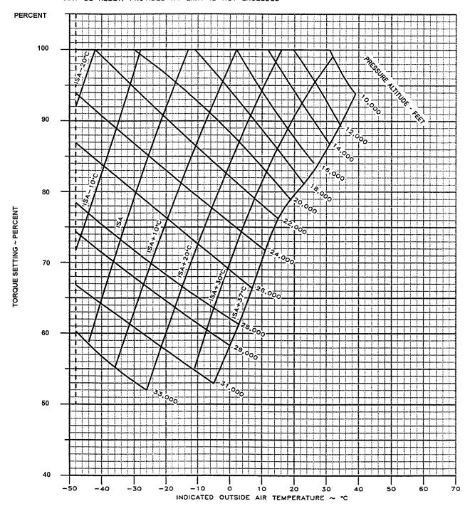
Figure 7A-55. Maximum Cruise Power, 1700 RPM
