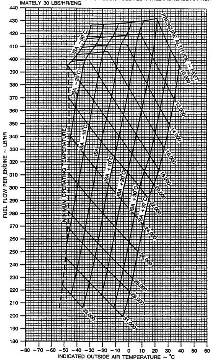
Figure 7A-68. Fuel Flow at Normal Cruise Power, 1800 RPM
