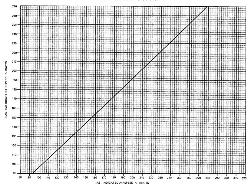
Figure 7A-8. Airspeed Calibration – Alternate System
