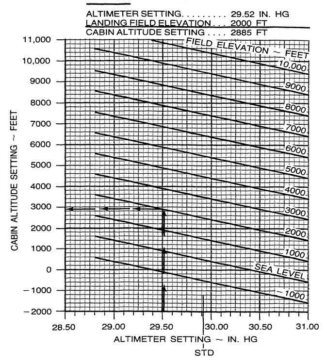
Figure 7A-103. Pressurization Controller Setting for Landing
