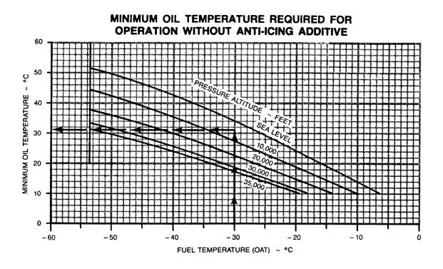
Figure 5-2. Oil/Fuel Temperature Graph
