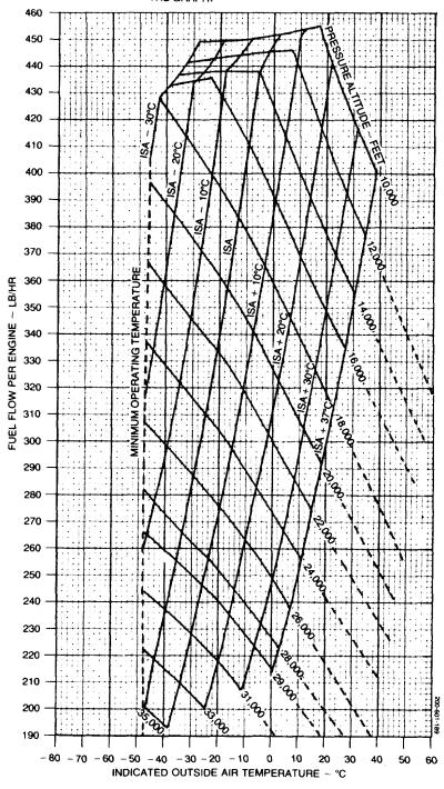
Figure 7-70. Fuel Flow at Maximum Cruise Power - 1900 RPM
