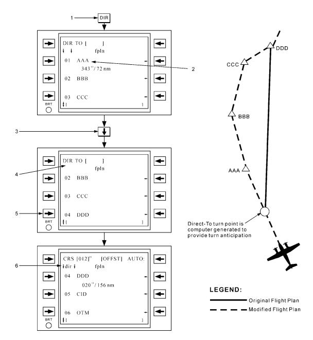
Figure 3C-47. Direct-To a Flight Plan Waypoint
