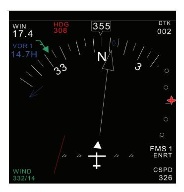
Figure 3C-11. HSI ARC Format (Off Display CRS, HDG, and Bearing)
