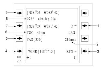
Figure 3C-67. Alternate Flight Plan Leg A Page
