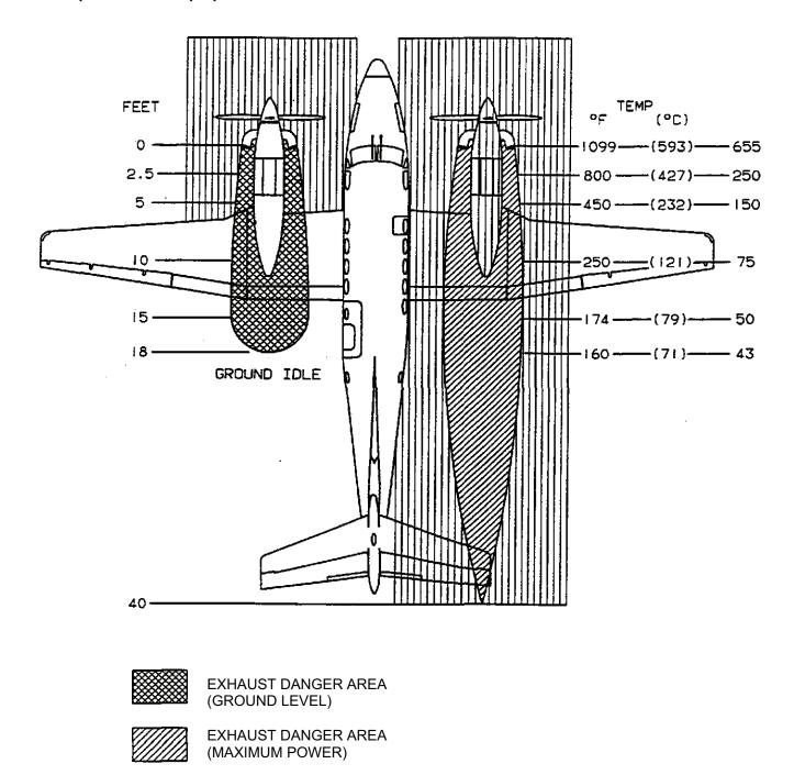
Figure 2-5. Exhaust and Propeller Danger Areas
