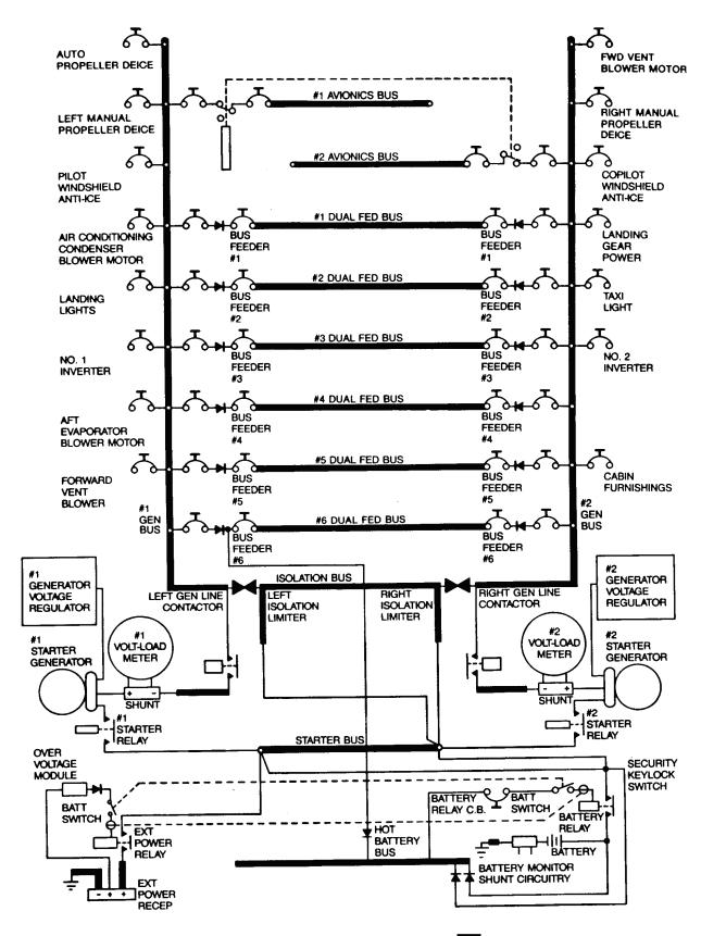
Figure 2-28. DC Electrical System Schematic T2 (Sheet 2 of 2)
