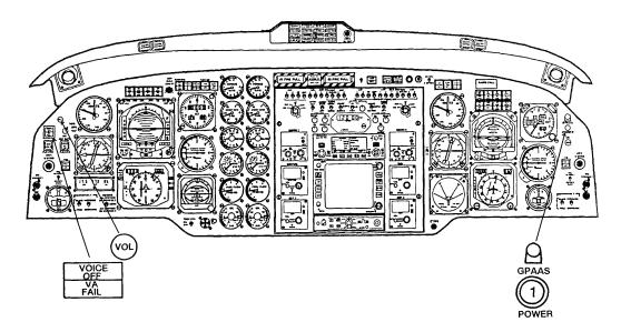
Figure 3C-149. Ground Proximity Altitude Advisory System Controls and Indicator
