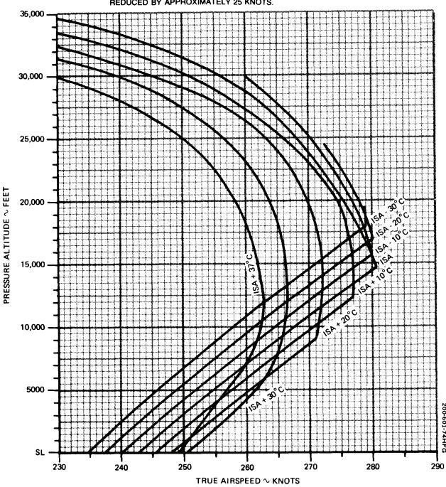
Figure 7-57. Recommended Cruise Speeds – 1800 RPM
