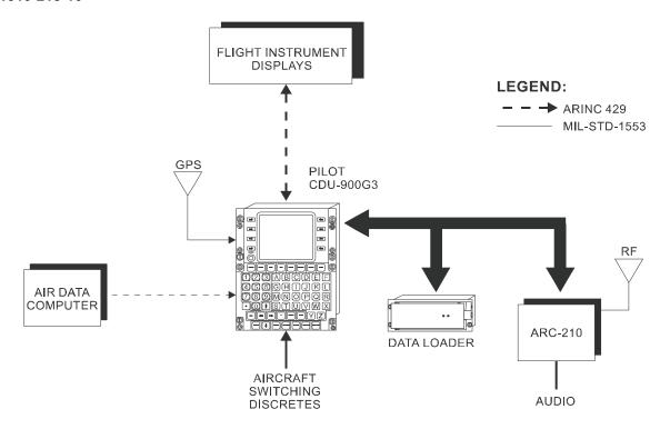
Figure 3C-22. FMS-800 Simplified Diagram
