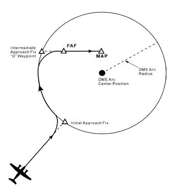
Figure 3C-93. DME Arc Flight Path
