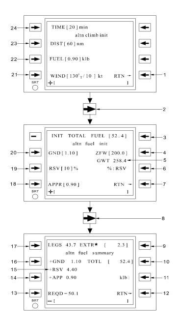
Figure 3C-66. Alternate Flight Plan Init and Fuel Pages
