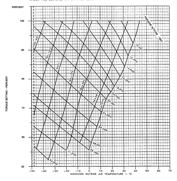
Figure 7A-43. Normal Cruise Power, 1700 RPM
