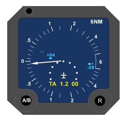
Figure 3C-156. No-Bearing Message Operational Situation
