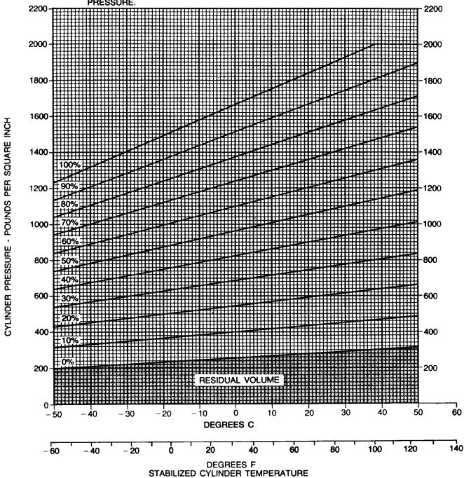
Figure 2-24. Oxygen System Servicing Pressure Chart
