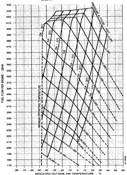
Figure 7-59. Fuel Flow at Recommended Cruise Power – 1800 RPM
