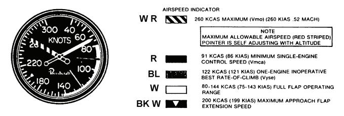
Figure 5-1. Instrument Markings and Operating Limits C (Sheet 7 of 8)
