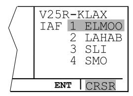
Figure 3-58. Selecting the Initial Approach Fix
