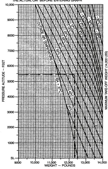
Figure 7A-16. Takeoff Weight to Achieve Positive One-Engine-Inoperative Climb at Lift-Off, Flaps APPROACH
