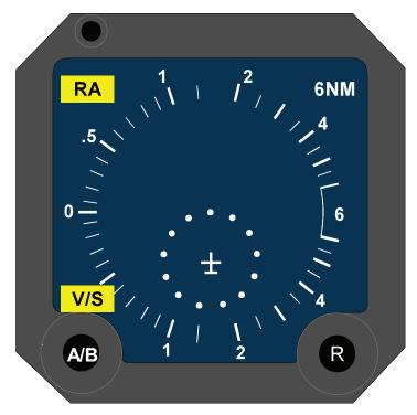
Figure 3C-158. Vertical Speed Indicator Failure
