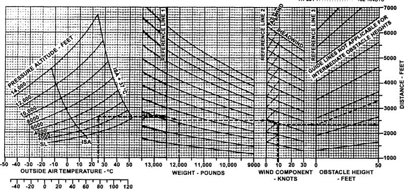
Figure 7-22. Accelerate – Stop Distance – Flaps 40%
