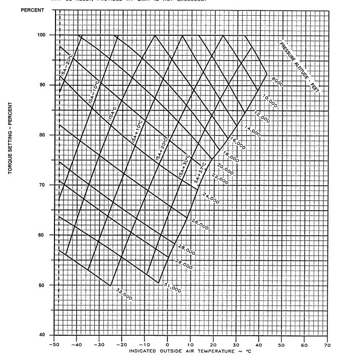
Figure 7A-79. Maximum Cruise Power, 1800 RPM
