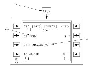
Figure 3C-83. Discontinuity in the Flight Plan
