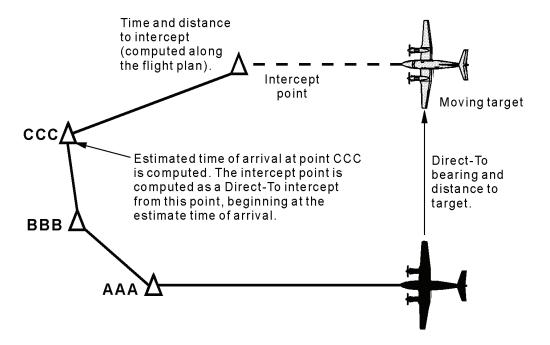
Figure 3C-103. Future Intercept Geometry Alternate Intercept Solution
