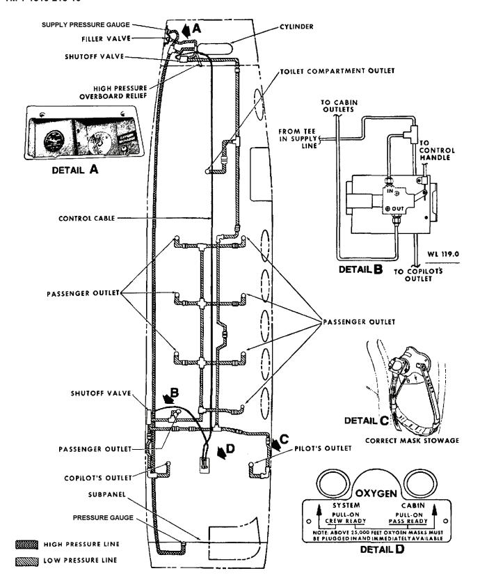
Figure 2-25. Oxygen System C (Sheet 1 of 2)
