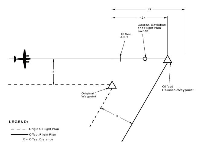
Figure 3C-54. Normal Parallel Offset Positions
