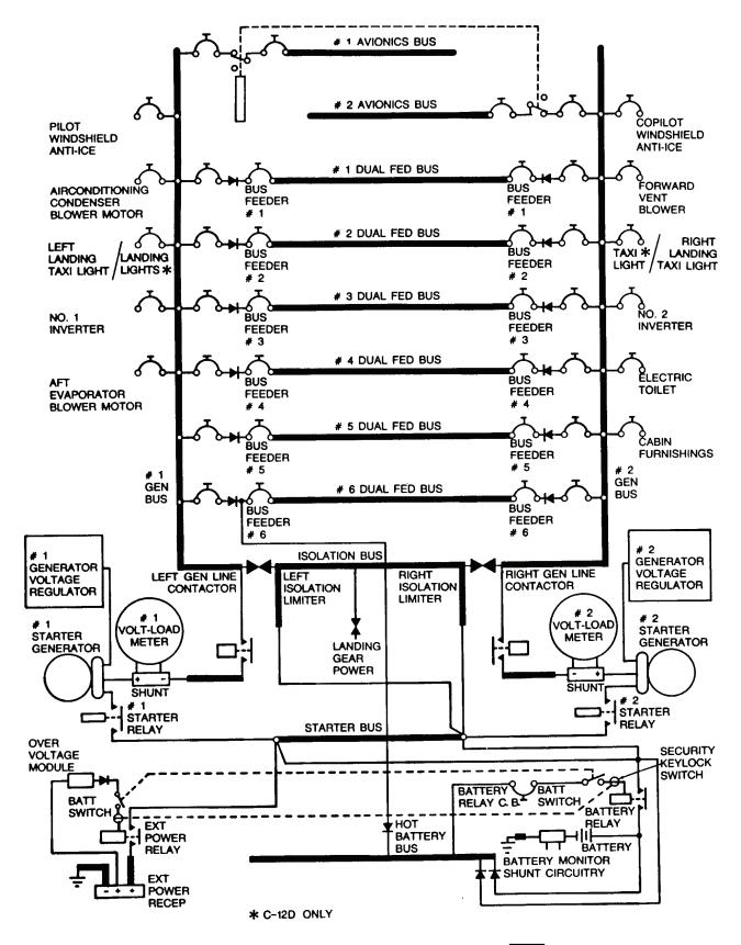
Figure 2-27. DC Electrical System Schematic C D1
