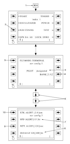
Figure 3C-30. Navigation Configuration Page Access and Functions
