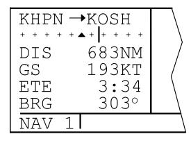
Figure 3-10. NAV 1 Page (Flight Plan Operation)
