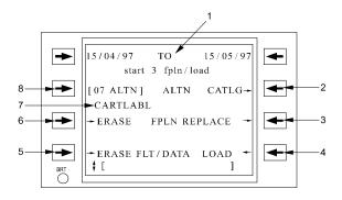
Figure 3C-29. Start 3 Flight Plan/Load Page
