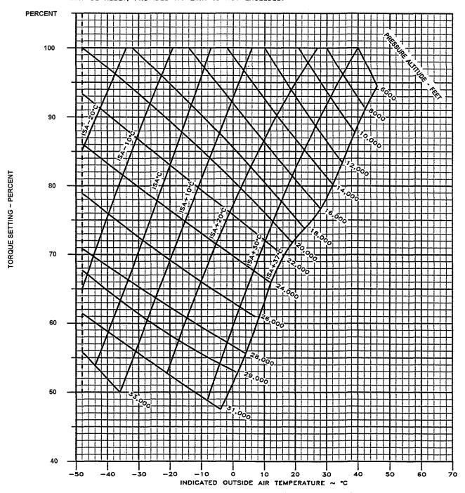
Figure 7A-67. Normal Cruise Power, 1800 RPM
