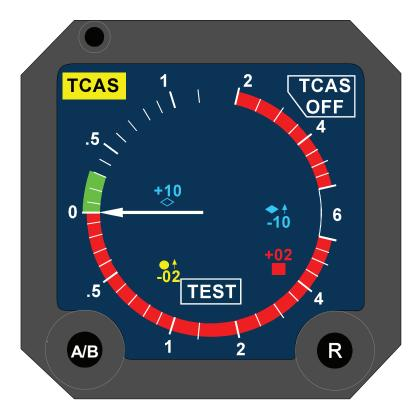
Figure 3C-159. TCAS System Test
