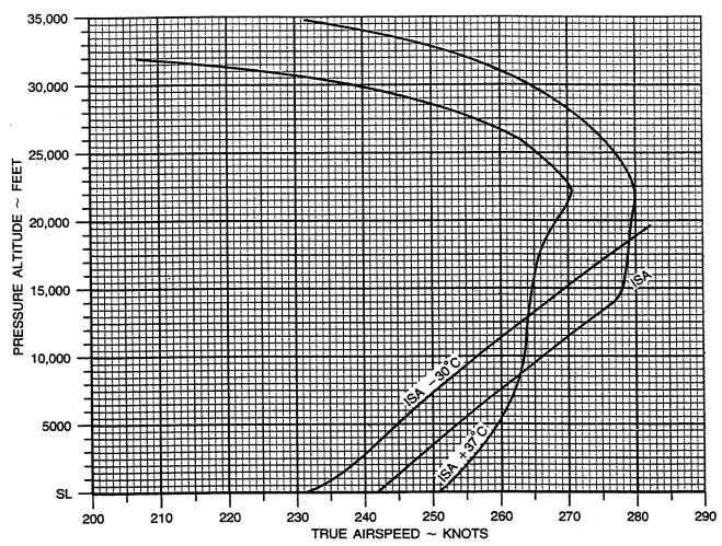
Figure 7A-66. Normal Cruise Speeds, 1800 RPM
