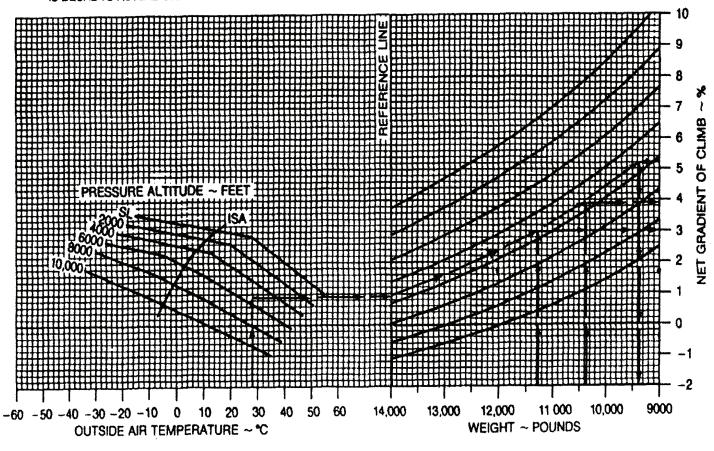
Figure 7A-24. Net Gradient of Climb, Flaps UP
