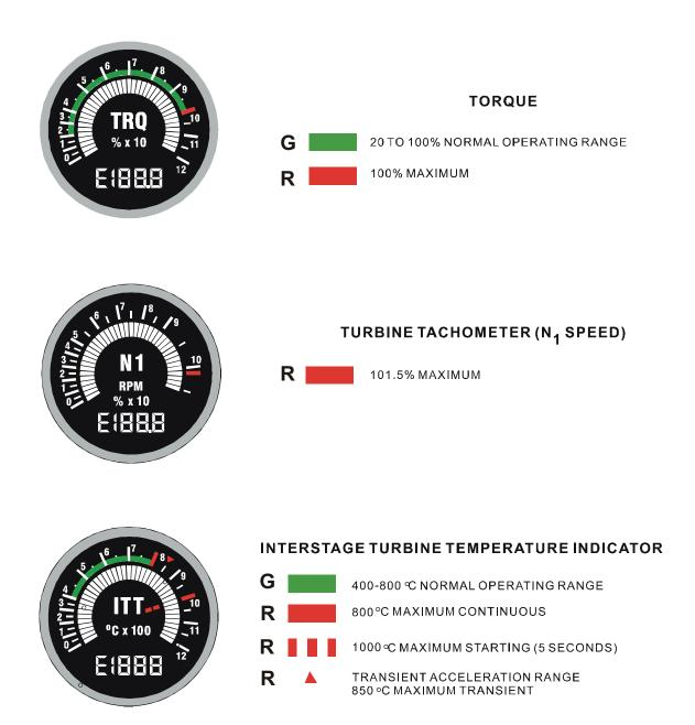
Figure 5-1. Instrument Markings and Operating Limits T1 T2 (Sheet 3 of 7)
