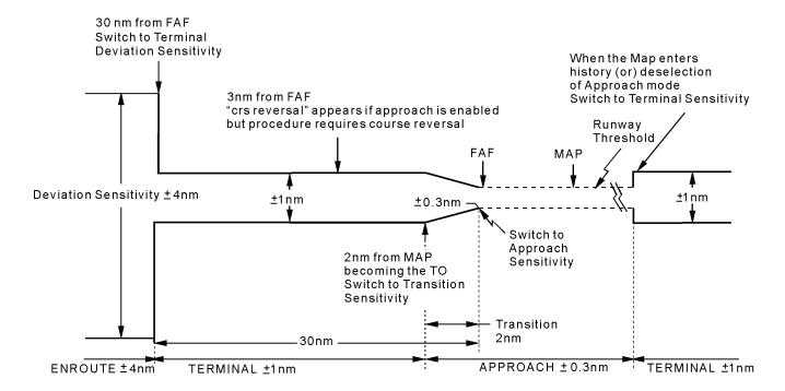
Figure 3C-92. Published GPS Approach Scaling and Sequencing
