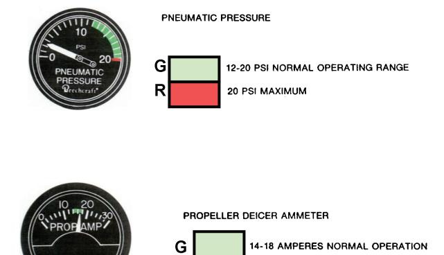
Figure 5-1. Instrument Markings and Operating Limits (Sheet 5 of 7)
