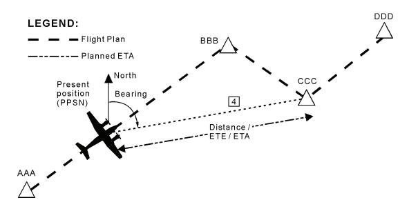
Option 4: PPSN DIRECT to CCC (present position direct to flight plan waypoint)
