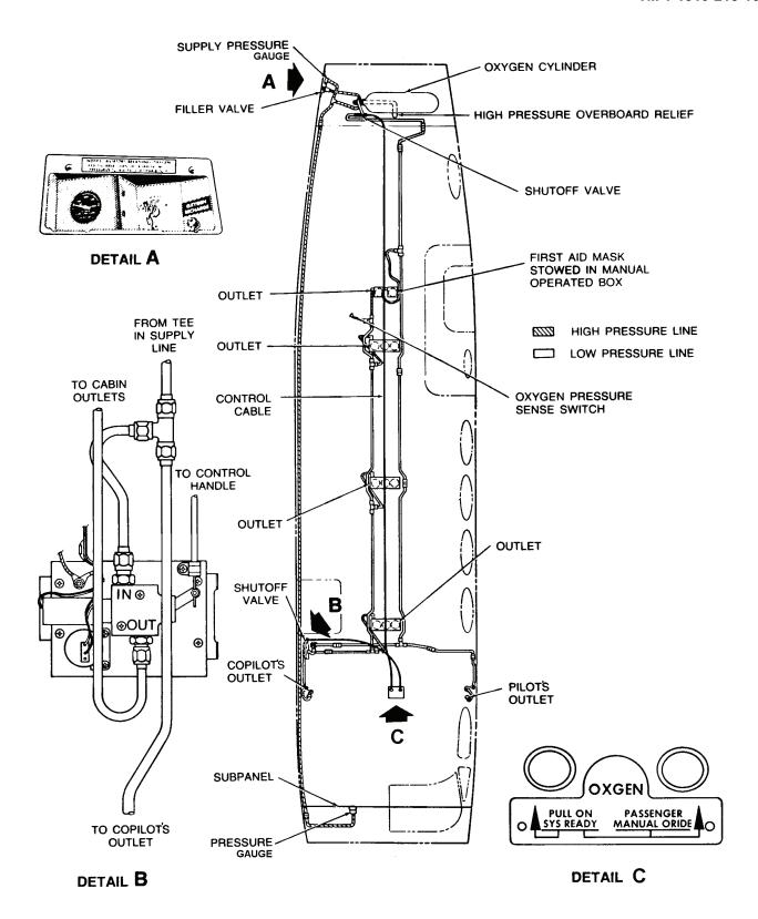
Figure 2-25. Oxygen System D T (Sheet 2 of 2)
