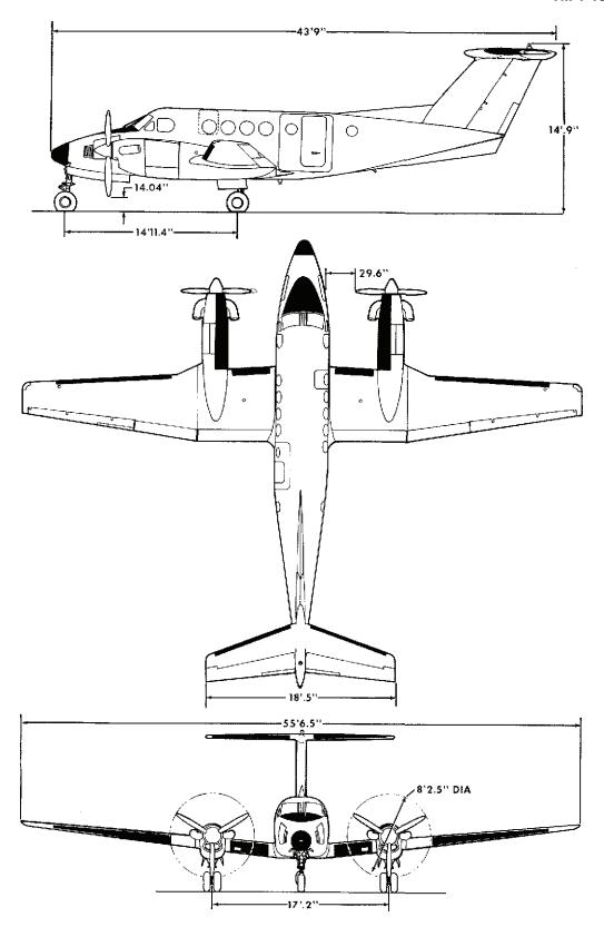
Figure 2-3. Principal Dimensions D T (Sheet 2 of 2)
