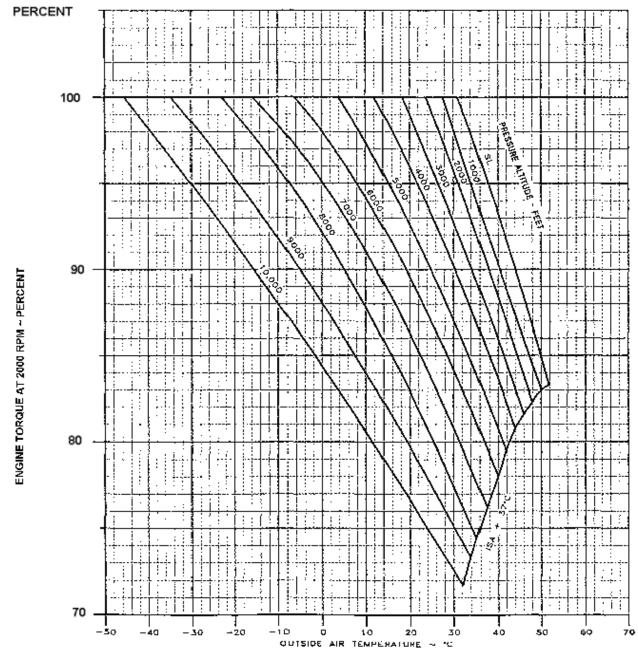
Figure 7A-17. Minimum Takeoff Power at 2000 RPM With Ice Vanes Retracted (65 Knots)
