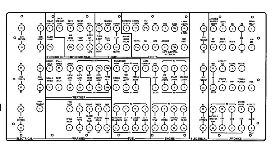
Figure 2-16. Overhead Circuit Breaker Panel D7 (Sheet 2 of 4)
