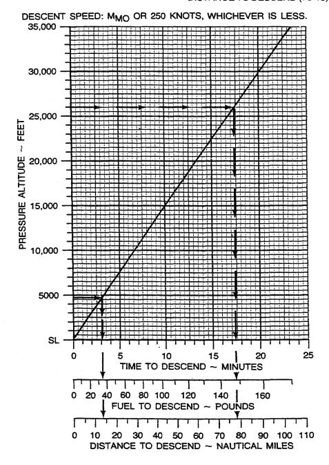
Figure 7A-105. Time, Fuel, and Distance to Descend
