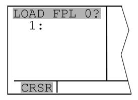
Figure 3-41. Storing 0 As A Numbered Flight Plan
