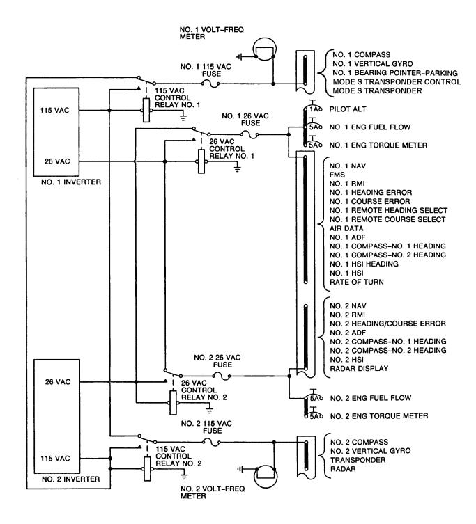
Figure 2-29. AC Electrical System Schematic Diagram T (Sheet 3 of 3)
