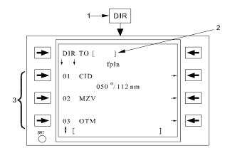
Figure 3C-46. Direct-To Line Select Key
