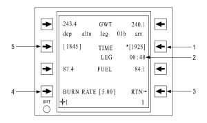
Figure 3C-68. Alternate Flight Plan Leg B Plan
