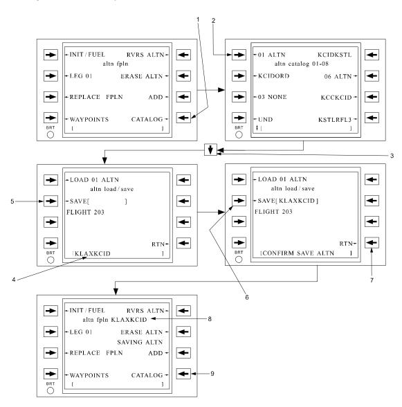
Figure 3C-70. Alternate Flight Plan Load/Save Page Access
