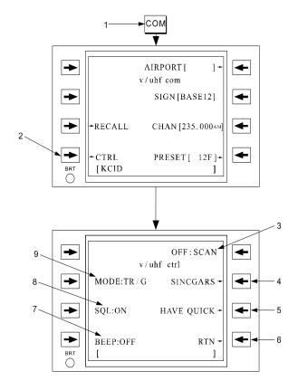
Figure 3C-129. V/UHF Control Functions
