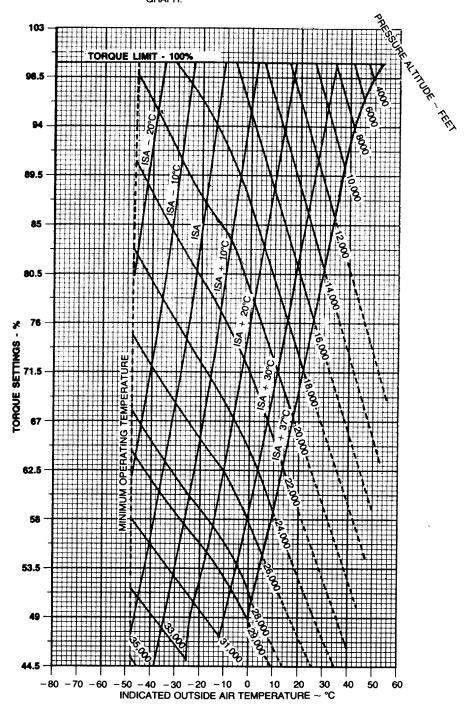
Figure 7-47. Recommended Cruise Power - 1700 RPM
