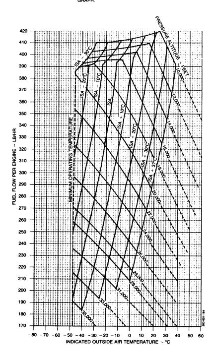
Figure 7-48. Fuel Flow at Recommended Cruise Power – 1700 RPM
