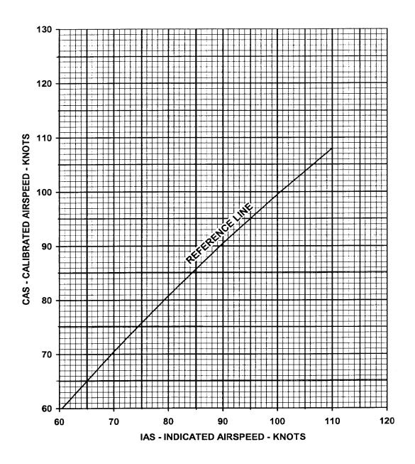
Figure 7-13. Airspeed Calibration – Normal System – Ground Roll
