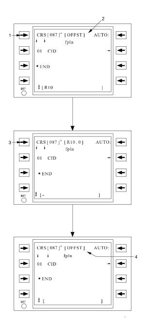
Figure 3C-52. Entering and Deleting Parallel Course Offsets
