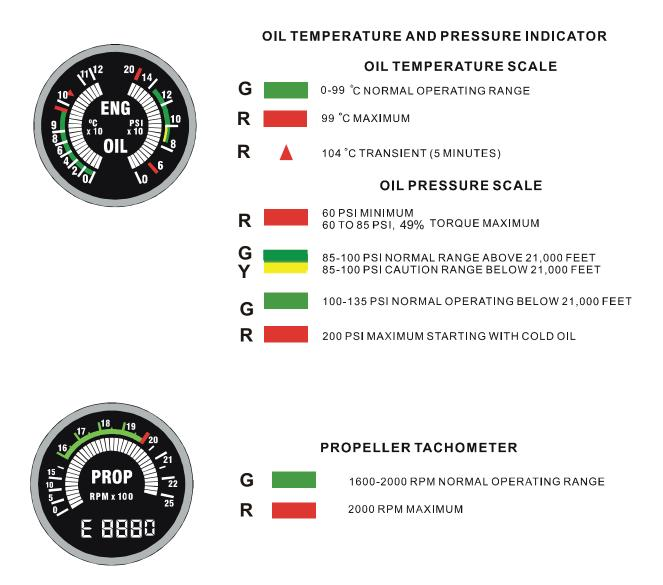
Figure 5-1. Instrument Markings and Operating Limits T1 T2 (Sheet 4 of 7)
