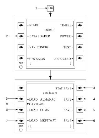
Figure 3C-137. Data Loader Page Access and Usage
