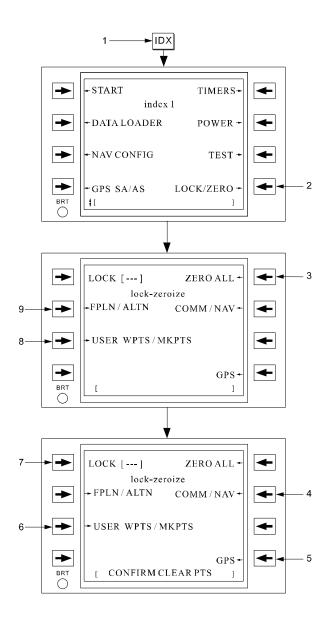
Figure 3C-142. Zeroizing or Locking Up System
