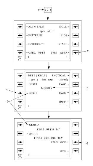
Figure 3C-86. Working Copy Approach Definition
