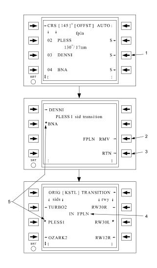
Figure 3C-81. Active Flight Plan SID/STAR Procedure
