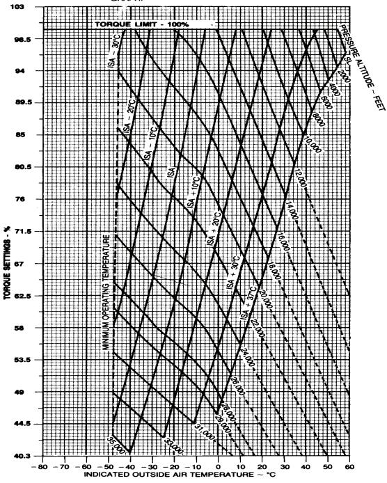
Figure 7-58. Recommended Cruise Power - 1800 RPM
