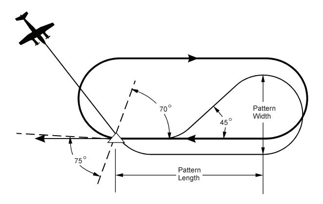
Figure 3C-75. Parallel Entry Into a Holding Pattern
