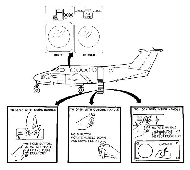
Figure 2-11. Cabin Door and Cabin Emergency Hatch C
