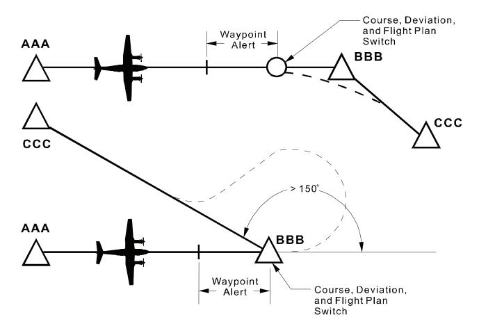
Figure 3C-38. Lateral To-To Course Transitions with Automatic Sequencing
