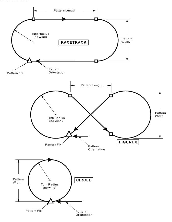
Figure 3C-99. MFP Geometry Definitions
