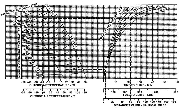
Figure 7-29. Service Ceiling – One Engine Inoperative
