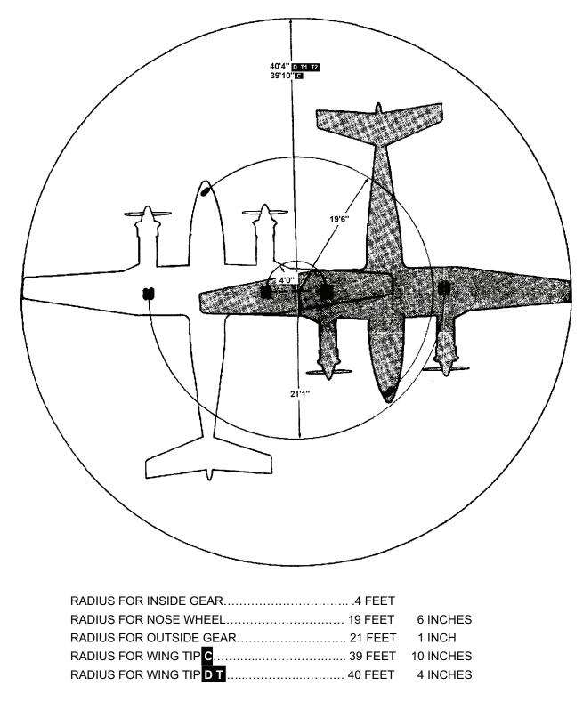
TURNING RADII ARE PREDICATED ON THE USE OF PARTIAL BRAKING ACTION AND DIFFERENTIAL POWER.
