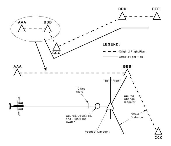
Figure 3C-51. Parallel Course Offset Geometry
