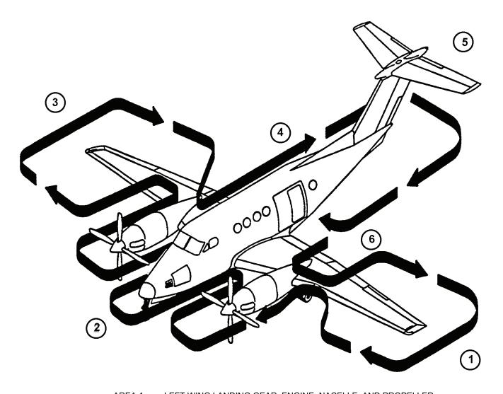
AREA 1 LEFT WING LANDING GEAR, ENGINE, NACELLE, AND PROPELLER
