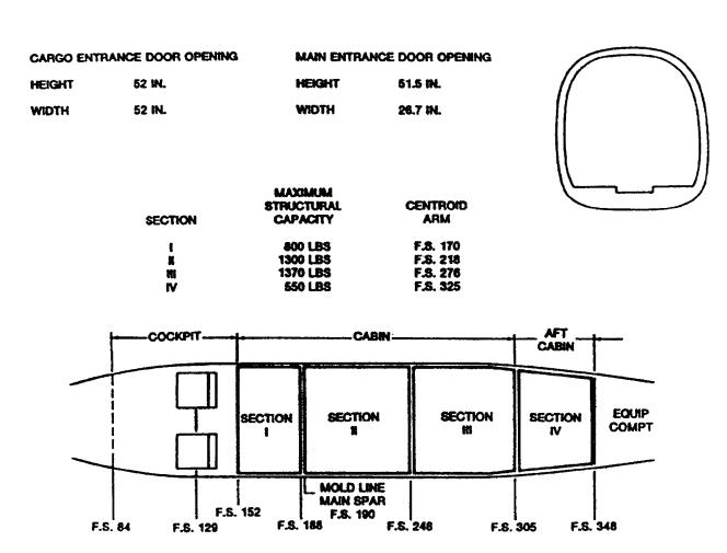
Figure 6-6. Cargo Loading T2 (2 of 2)
