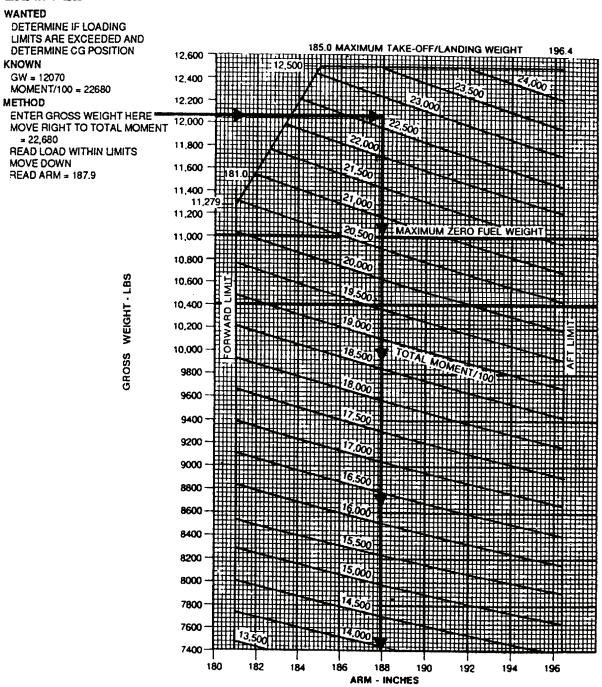
Figure 6-7. Center of Gravity Limitations
