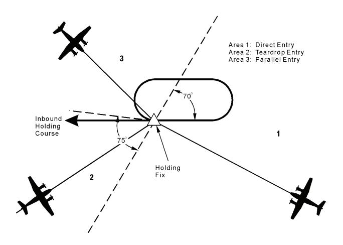
Figure 3C-72. Required Entry Methods
