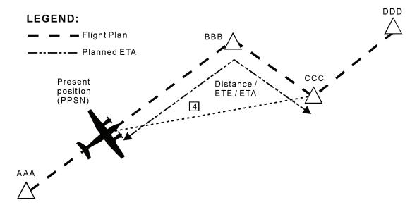
Option 4: PPSN VIA FPLN to CCC (present position through flight plan to flight plan waypoint)
