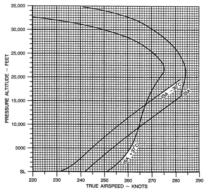
Figure 7A-78. Maximum Cruise Speeds, 1800 RPM
