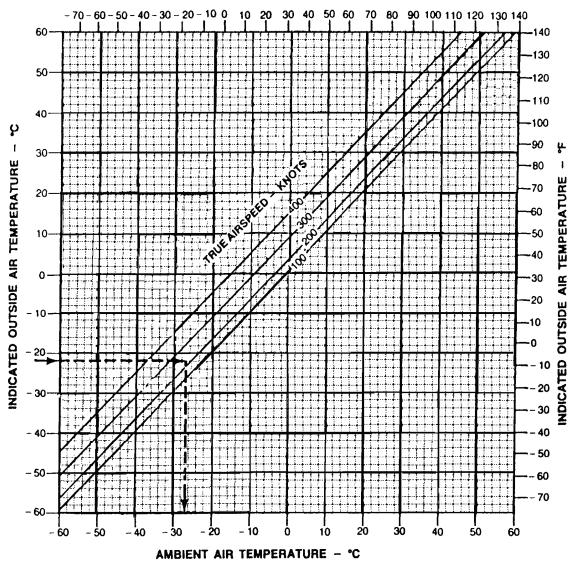
Figure 7-10. Temperature Conversion/Correction for Compressibility
