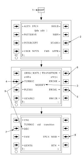
Figure 3C-82. Working Copy SID/STAR Procedure
