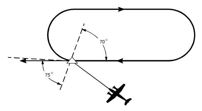
Figure 3C-73. Direct Entry Into a Holding Pattern
