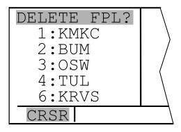
Figure 3-40. Deleting a Flight Plan
