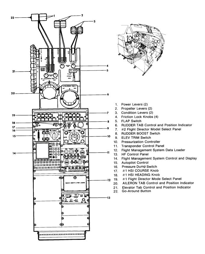
Figure 2-9. Control Pedestal D2 (Sheet 1 of 3)
