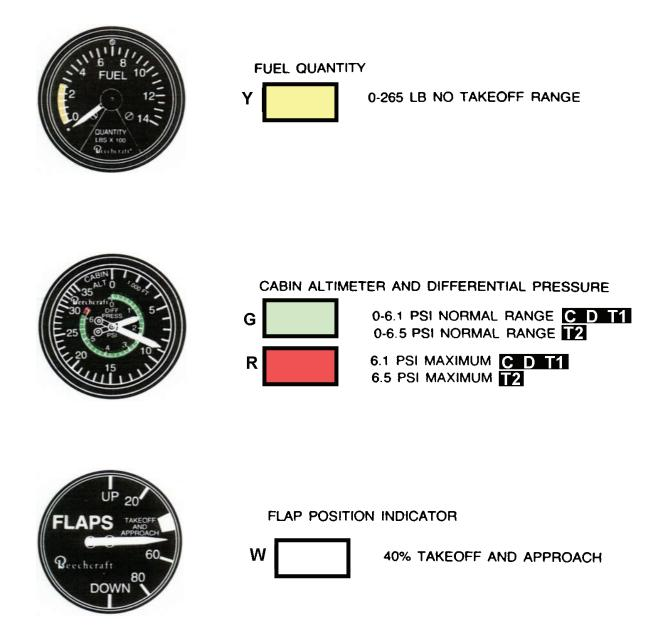
Figure 5-1. Instrument Markings and Operating Limits (Sheet 6 of 7)
