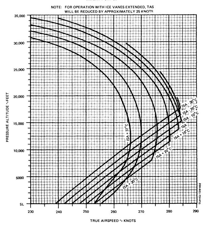
Figure 7-68. Maximum Cruise Speeds - 1900 RPM
