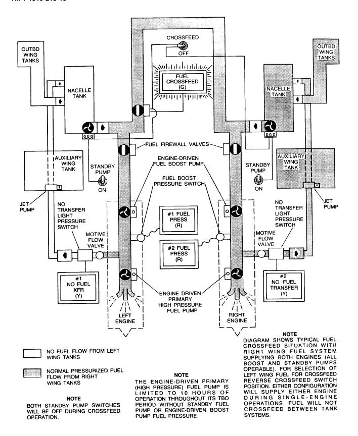
Figure 2-21. Crossfeed Fuel Flow
