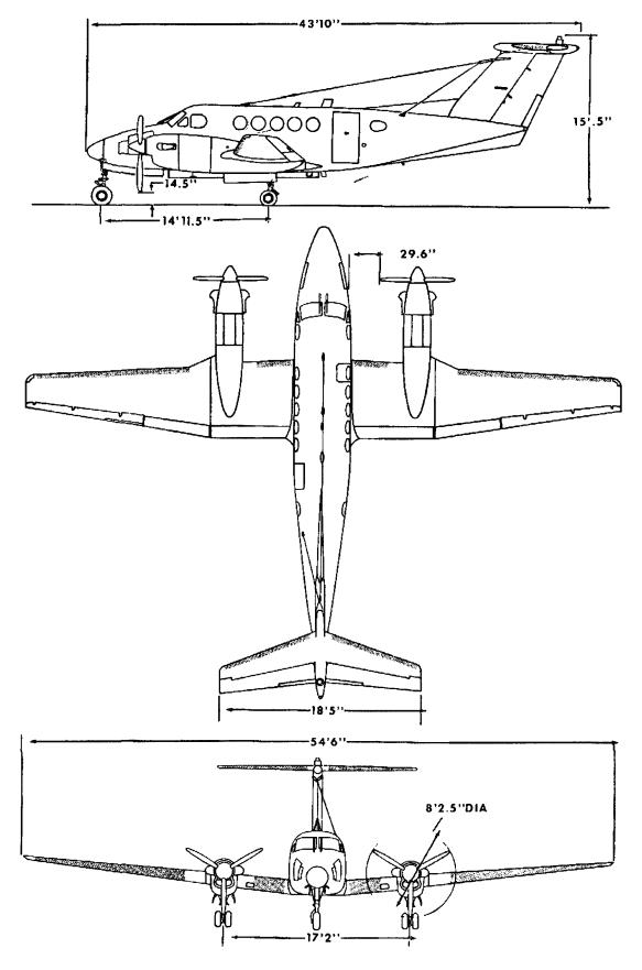
Figure 2-3. Principal Dimensions **C** (Sheet 1 of 2)
