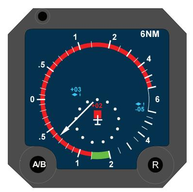
Figure 3C-154. Corrective RA Operational Situation
