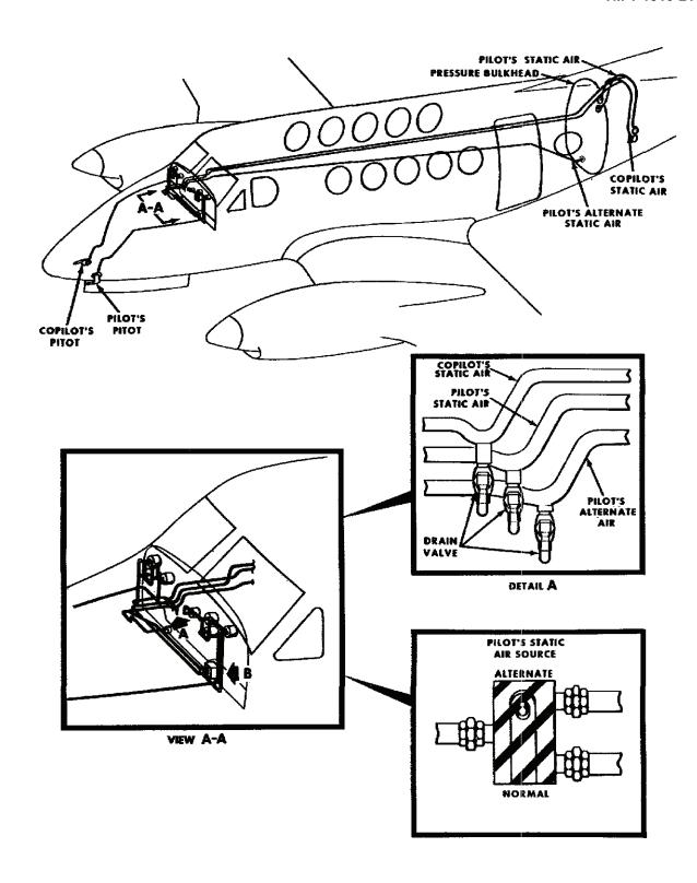
Figure 2-31. Pitot and Static System
