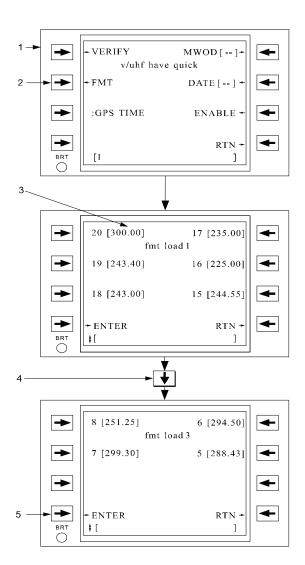
Figure 3C-131. V/UHF FMT List Selection and Loading
