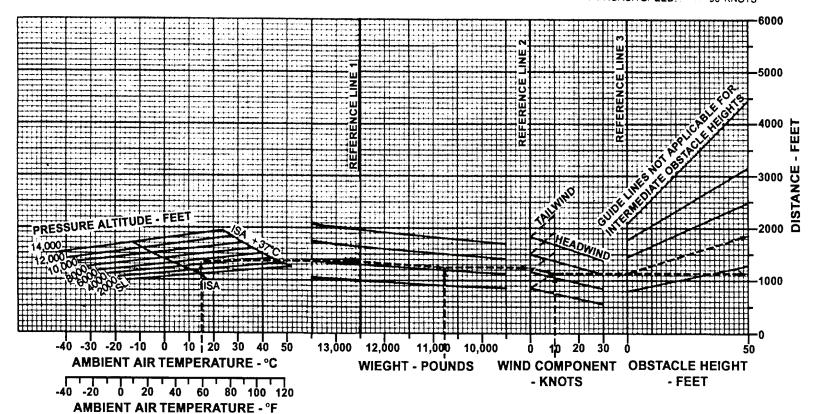
Figure 7-34. Landing Distance With Propeller Reversing – Flaps 40% MODEL: C-12 CD DATE: 11 JANUARY 1988 DATA BASIS: ESTIMATED
