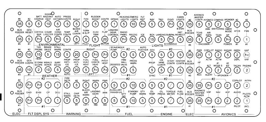
**Figure** 2-16. Overhead Circuit Breaker Panel **71** (Sheet 4 of 4)
