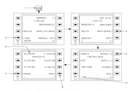
Figure 3C-130. UHF MWOD List Selection and Loading
