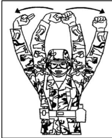
Figure A-24. Disconnect auxiliary power unit (day)
