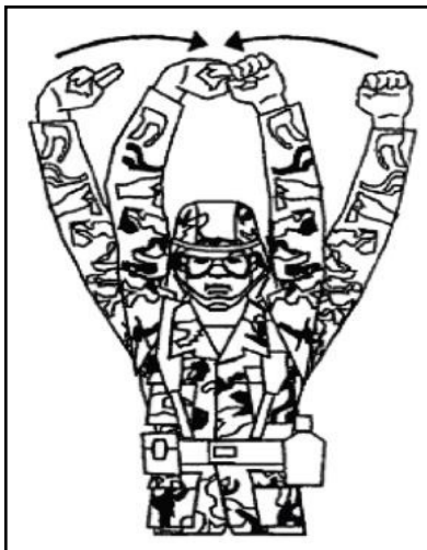
Figure A-23. Connect auxiliary power unit (day)
