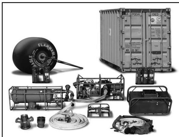
Figure 2-3. Advanced aviation forward area refueling system
