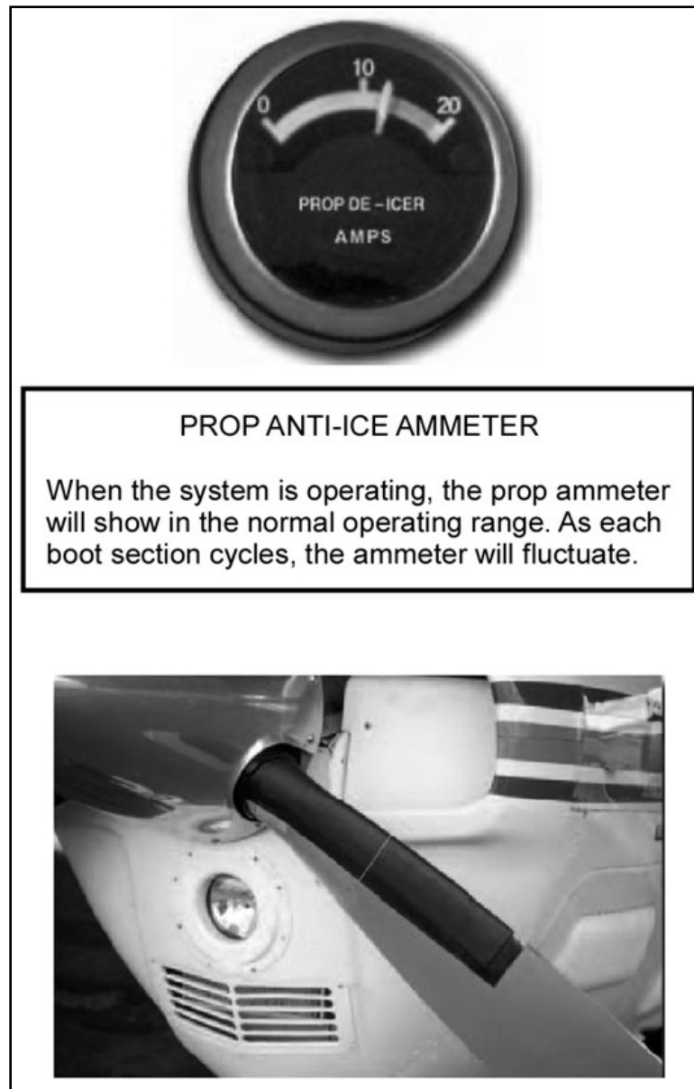
Figure 8-5. Propeller ice control
